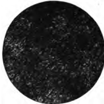
Fig. 22. Martensite Structure in a Fine-grained Steel
